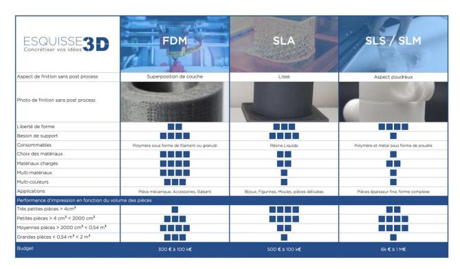
FDM: fused deposit filament; SLA (DLP): stereolithography (Digital Light Processing), SLS: selective laser sintering / SLM: selective laser melting
