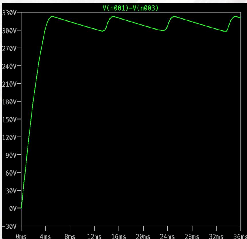
$R = 1 \text{ k}\Omega$ ,  $U_{\text{moy}} = 315 \text{ V}$
